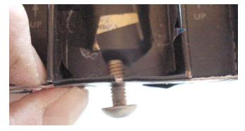
Put the bolt through the hole and screw the nut on it inside to make sure the nut will be aligned with the hole. Put lots of glue on the stack of parts with the cutouts,, and being careful not to bend your clicker, slide it over the nut and put the clamp on it.
