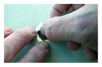
The hole will probably be a somewhere around .15mm if you're using a #10 needle, a little bigger than .2mm if you're using a common pin.. The ideal size for this camera is .22, but in my opinion, a little smaller is better. (I typically use .15mm pinholes)
