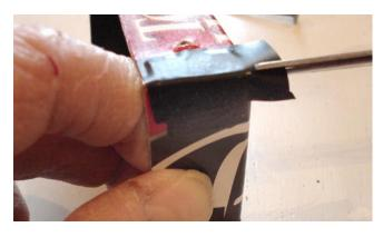
Then fold in these flaps, one parallel to the side and one parallel to the top. The front corners are a potential source of a light leak, so you want to make sure they get covered.
