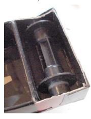
It will probably take four or five pieces to go completely around the dowel. Be careful not to tape the winder collar to the top of the camera.
