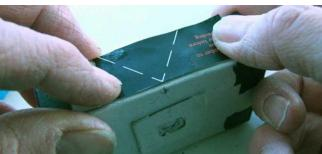
Glue the exposure guide to the back of the camera. (If your pinhole was significantly different from .20mm, we'll provide other exposure guides later on.)
