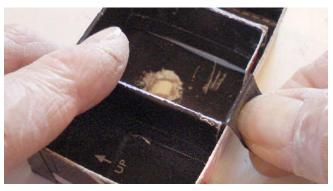
Cover the sides of the interior divider with tape. Make sure its smooth without any wrinkles or bumps. The film will ride over this surface when you advance and rewind the film.
