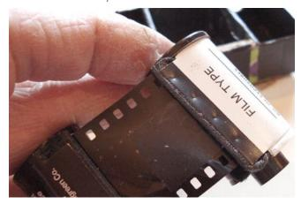
Place the film and take-up cassettes into the camera. Adjust it slightly so the clicker extend through the sprocket holes. You may have to put the winder into the winding hole and advance it a bit to tighten up the film.
