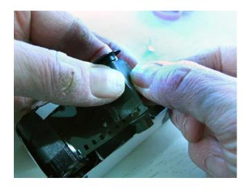
Place the empty film cassette over the take-up spool. The camera should be light tight, but just in case there's a bit of a leak through the winding hole, this will protect your exposed film. It's not necessary to close the bottom of the cassette.
